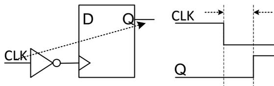
This will increase the delay through the divider chain. As such the user should be even more aware of the timing behaviour.
