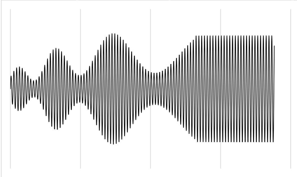
Both of the above waveforms can produce pulses which are much shorter than the crystal period. This can (actually: *will*) upset any downstream logic.
