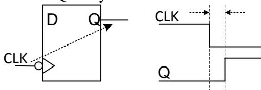
As a single delay this is not too bad. However in a long chain of dividers this delay can add up:
