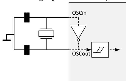
The oscillation is not a nice square wave but a sine signal. In order to use this signal the oscillator output is passed through a Schmitt trigger.
