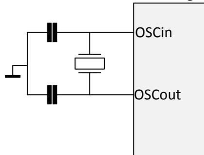
Inside the controller is an inverting amplifier which makes that the circuit start oscillating. This is a slightly more accurate picture:
