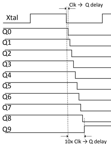
The last stage of the delay chain is used to switch off the input to the dividers and to pass the crystal clock to the output. This produces a clean clock *then and only then* when the delay chain is shorter than the low period of the incoming crystal clock.
